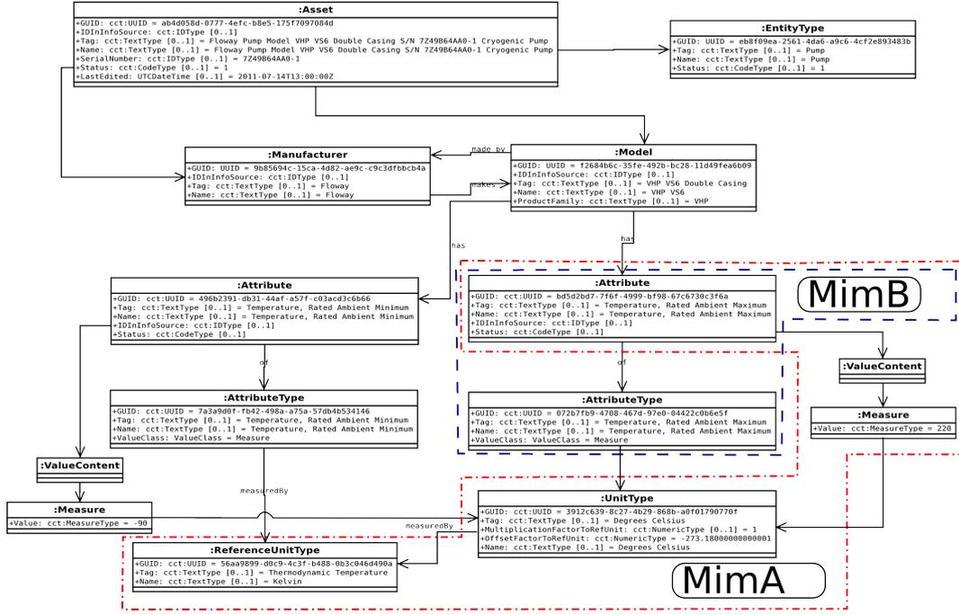
Figure 2: MIMOSA CCOM: Ambient Temperature Range
