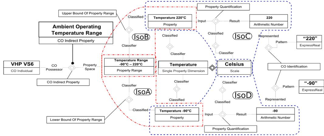
Figure 3: ISO 15926: Ambient Temperature Range
